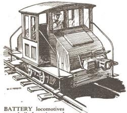
BATTERY locomotives were built for mine and tunnel work
